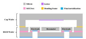
Figure 1: MEMS structure after vacuum WLP with eutectic bonding.
